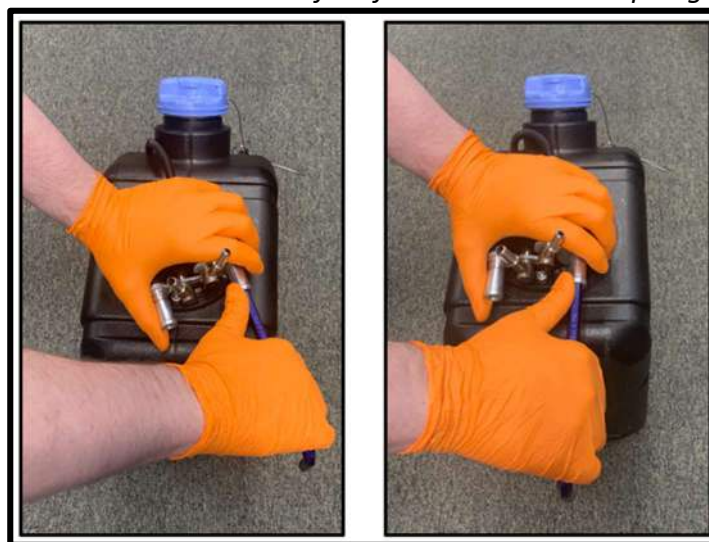
Figure 2.12 Installation of Head Unit
